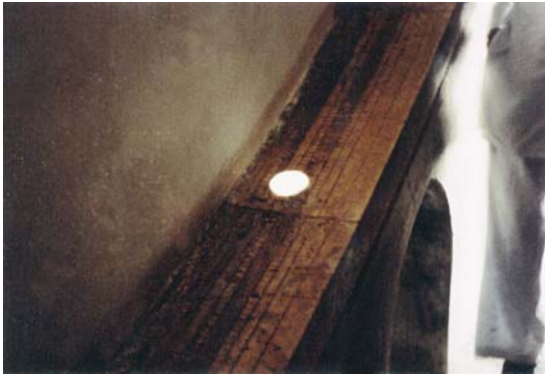
Astronomical Instruments in India. Plate 5 Image of the sun projected on the Śaṣṭāmśa-yantra in Jai Singh's observatory at Jaipur.
